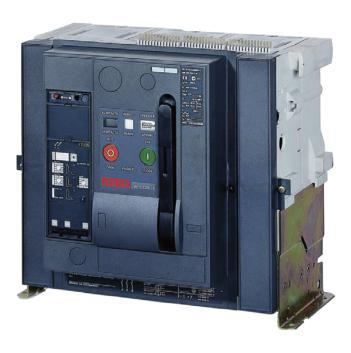
Techna's high performance Atec Air Circuit Breakers provide protection and switching for electrical equipment from 630A to 6300A. With 3 different model sizes, the Atec ACBs are available as a fixed or withdrawable design.
